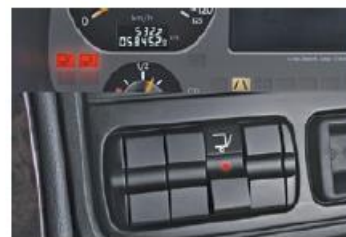
Trucks with an electrical preparation following ETMA with a prefitted display light in the driver's cabin.
